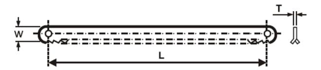
46.2 Confirming to IS: 2594 Compliance: 46.3 Length 'L': 300 mm Width 'W': 46.4 12.5 mm 46.5 Thickness 'T': 0.63 mm 46.6 TPI: 18 46.7 Material: HSS M2 46.8 Finish: Milling Teeth 46.9 Hardness: 62-65 HRC 46.10 The blades coated with a suitable preservative or paint. 46.11 Packet consisting of 100 Blades.
