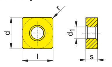
164.2 Type of Insert: Milling164.3 Number of cutting edges: 8
