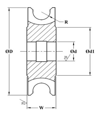
100.2 Compliance: Confirming to IS: 6322 - 1982 Diameter 'ØD': 100.3 Ø63.00 js16 (±0.950) 100.4 Bore Diameter 'Ød': Ø27.0 H7 (+0.021/ -0.0) 100.5 Diameter 'Ød1': 34.00 mm 100.6 Radius 'R': 2.5.00 mm 100.7 Cutter Width 'W': 10.00 mm 100.8 Material: HSS-M2 100.9 Finish: Milled/ Ground 760 HV to 900 HV 100.10 Hardness:
