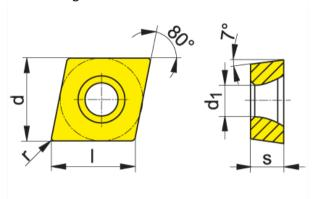
76.2 Type of Insert: Turning 9 mm 76.3 Size: 76.4 0.4 mm **Corner Radius:** 76.5 Length (I): 9.7 mm 76.6 Width (d): 9.5 mm 76.7 Thickness (s): 3.97 mm 76.8 Hole Size (d1): 2.80 mm
