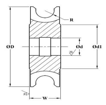
104.2 Compliance: Confirming to IS: 6322 - 1982 104.3 Diameter 'ØD': Ø80.00 js16 (±0.950) Bore Diameter 'Ød': Ø27.0 H7 (+0.021/ -0.0) 104.4 104.5 Diameter 'Ød1': 41.00 mm 104.6 Radius 'R': 6.00 mm Cutter Width 'W': 104.7 24.00 mm 104.8 Material: HSS-M2 104.9 Finish: Milled/ Ground 104.10 Hardness: 760 HV to 900 HV 104.11 Surface Treatment: **Dual Finish**
