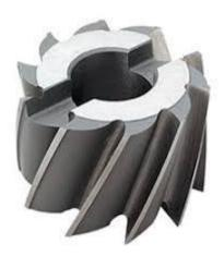
186.2 Diameter 40 mm 186.3 Width 32 mm 186.4 Bore 16 mm 186.5 Compliance: Confirming to IS BS 122 Part 1: 1989 186.6 Cutting Portion Material: HSS-M2 186.7 Finish: Milled flute 62 - 65 HRC 186.8 Hardness: 186.9 Surface Treatment: Sand Blast or Steam Blue finish
