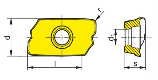
133.2 Type of Insert: Milling133.3 Number of cutting edges: 2133.4 Corner Radius (r): 0.80 mm
