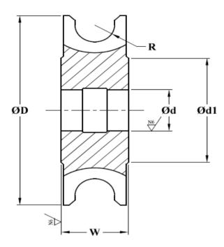
105.2 Compliance: Confirming to IS: 6322 - 1982 105.3 Diameter 'ØD': Ø80.00 js16 (±0.950) Bore Diameter 'Ød': Ø27.0 H7 (+0.021/ -0.0) 105.4 105.5 Diameter 'Ød1': 41.00 mm Radius 'R': 105.6 8.00 mm 105.7 Cutter Width 'W': 32.00 mm 105.8 Material: HSS-M2 105.9 Finish: Milled/ Ground
