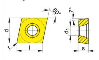
86.2 Type of Insert: Turning 86.3 Size: 9 mm 86.4 Corner Radius: 0.8 mm 86.5 Length (I): 9.7 mm 86.6 Width (d): 9.5 mm Thickness (s): 86.7 3.97 mm 86.8 Hole Size (d1): 4.40 mm
