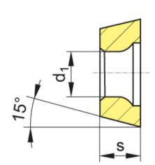
Type of Insert: Milling 134.2 134.3 Number of cutting edges: Corner Radius: 134.4 0.8 mm 134.5 Length (I): 9.52 mm 134.6 Width (d): 9.52 mm 134.7 Thickness (s): 3.97 mm 134.8 Hole Size (d1): 4.40 mm
