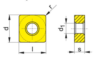
163.2 Type of Insert: Milling163.3 Number of cutting edges: 8163.4 Corner Radius (r): 0.80 mm
