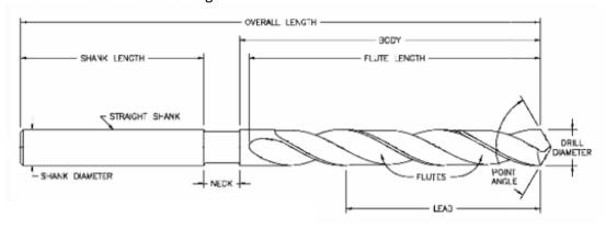
43.2 Compliance: Confirming to IS: 5101 - 1991 43.3 Drill Diameter 'ØD': Ø1.0 mm to Ø 13.0 mm
