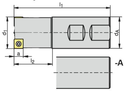
161.2 Type of Cutter: Right hand 161.3 Diameter (d1): 20.0 mm 161.4 Diameter (dA): 20.0 mm 161.5 Length (I1): 200.0 mm 161.6 Length (I2): 40.0 mm 161.7 Max RPM: 10500 161.8 Number of Pockets (Z): 2 Numbers
