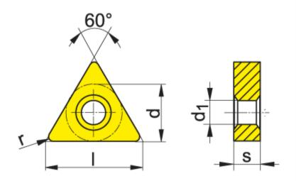
87.2 Type of Insert: Turning 87.3 Size: 16 mm 87.4 0.8 mm **Corner Radius:** 87.5 Length (I): 16.50 mm 87.6 Width (d): 9.52 mm Thickness (s): 87.7 4.76 mm 87.8 Hole Size (d1): 3.81 mm
