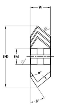
116.2 Compliance: Confirming to IS: 6325 - 1971 116.3 Diameter 'ØD': Ø50.00 js16 (± 0.950) 116.4 Bore Diameter 'Ød': Ø16.0 H7 (+0.021/ -0.0)
