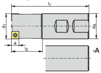
160.2 Type of Cutter: Right hand 160.3 Diameter (d1): 16.0 mm 160.4 Diameter (dA): 16.0 mm 160.5 Length (I1): 165.0 mm 160.6 Length (I2): 32.0 mm 160.7 Max RPM: 14800 160.8 Number of Pockets (Z): 2 Numbers
