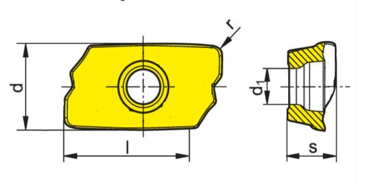
132.2 Type of Insert: Milling132.3 Number of cutting edges: 2132.4 Corner Radius (r): 0.80 mm
