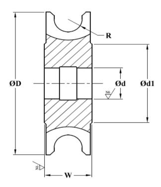
103.2 Compliance: Confirming to IS: 6322 - 1982 103.3 Diameter 'ØD': Ø63.00 js16 (±0.950) 103.4 Bore Diameter 'Ød': Ø27.0 H7 (+0.021/ -0.0) 103.5 Diameter 'Ød1': 34.00 mm 103.6 Radius 'R': 10 mm Cutter Width 'W': 40.00 mm 103.7 103.8 Material: HSS-M2 Milled/ Ground 103.9 Finish: 103.10 Hardness: 760 HV to 900 HV
