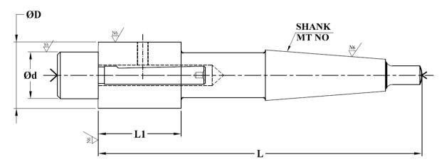
Compliance: Confirming to IS: 5710 - 1988 (Reaffirmed: 2002) 2.2 2.3 Diameter 'ØD': Ø18.00 z9 2.4 Overall Length 'L': 140.00 mm 2.5 Cutting Length 'L1': 25.00 mm 2.6 Pilot Diameter 'Ød': Ø9.00 e8 2.7 Shank: MT-2 2.8 **Cutting Portion Material:** HSS-M2 2.9 Finish: Milled/ Ground 2.10 Hardness 2.10.1 Cutting Portion: 760 HV to 900 HV 2.10.2 Shank Portion: 185 HV Min.
