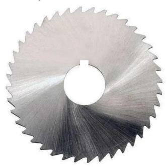
173.2 Compliance: Confirming to IS 5031-1992 Ø 75 mm ± 0.1 mm 173.3 Diameter: 173.4 Ø 27 mm ± 0.05 mm Inner Diameter: 173.5 Thickness: 3 mm ± 0.05 mm Coarse Pitch 32 173.6 No. of Teeth: 173.7 Hardness: 55 to 60 HRC 173.8 Material: **High Speed Steel** 173.9 Suitable Wooden/ Plastic/ Metal Box for storage.
