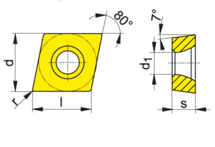
75.2 Type of Insert: Turning 75.3 Size: 6 mm 75.4 Corner Radius (r): 0.40 mm 75.5 Length (I): 6.40 mm 75.6 Width (d): 6.35 mm 75.7 Thickness (s): 2.38 mm 75.8 Hole Size (d1): 2.80 mm
