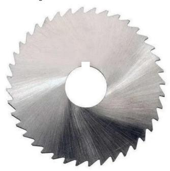
175.2 Compliance: Confirming to IS 5031-1992 Ø 80 mm ± 0.1 mm 175.3 Diameter: 175.4 Ø 27 mm ± 0.05 mm Inner Diameter: 175.5 Thickness: 4 mm ± 0.05 mm Coarse Pitch 32 175.6 No. of Teeth: 175.7 Hardness: 55 to 60 HRC 175.8 Material: **High Speed Steel**
