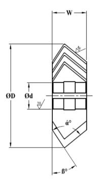
118.2 Compliance: Confirming to IS: 6325 - 1971 118.3 Diameter 'ØD': Ø63.00 js16 (± 0.950) 118.4 Bore Diameter 'Ød': Ø27.0 H7 (+0.021/ -0.0) 118.5 Cutter Width 'W': 18.00 mm 55° 118.6 Angle ' $\alpha$ ': 12° 118.7 Angle 'ß': Material: 118.8 HSS-M2 Milled/ Ground 118.9 Finish:
