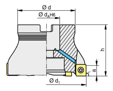
131.2 Type of Cutter: Right hand 131.3 Diameter (d1): 160.0 mm Diameter (d): 131.4 98.0 mm 131.5 Bore Diameter (da): 40.0 mm Thickness (h): 131.6 63.0 mm 131.7 Max RPM: 9800 131.8 Number of Pockets (Z): 14 Numbers
