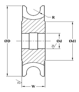
101.2 Compliance: Confirming to IS: 6322 - 1982 101.3 Diameter 'ØD': Ø63.00 js16 (±0.950) 101.4 Bore Diameter 'Ød': Ø27.0 H7 (+0.021/ -0.0) 101.5 Diameter 'Ød1': 34.00 mm 101.6 Radius 'R': 4.00 mm Cutter Width 'W': 16.00 mm 101.7 101.8 Material: HSS-M2 Milled/ Ground 101.9 Finish:
