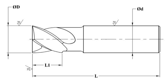
149.2 Compliance: Confirming to IS: 6352 - 1991 149.3 Diameter 'ØD': Ø14.0 e8 (-0.032/ -0.059) 149.4 Shank Diameter 'Ød': Ø12.0 h8 (+0.0/ -0.027) 149.5 Cutting Length 'L1': 26.0 mm 149.6 Overall length 'L': 83.0 mm Material: 149.7 HSS-M2
