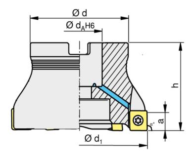
129.2 Type of Cutter: Right hand Diameter (d1): 80.0 mm 129.3 129.4 Diameter (d): 58.0 mm 129.5 Bore Diameter (da): 27.0 mm 129.6 Thickness (h): 50.0 mm 129.7 Max RPM: 7400 129.8 Number of Pockets (Z): 6 Numbers
