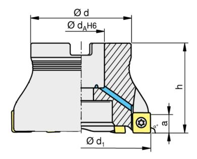
128.2 Type of Cutter: Right hand Diameter (d1): 50.0 mm 128.3 128.4 Diameter (d): 43.0 mm 128.5 Bore Diameter (da): 22.0 mm 128.6 Thickness (h): 40.0 mm Max RPM: 9800 128.7 128.8 Number of Pockets (Z): 4 Numbers
