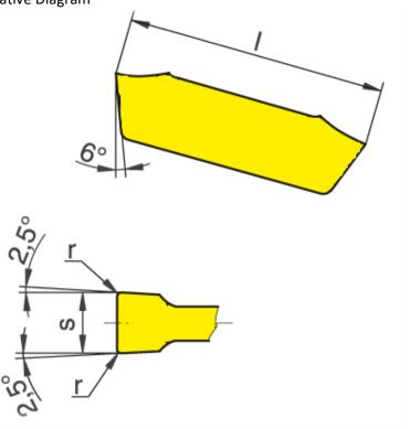
89.2 Type of Insert: Grooving 89.3 Size (S): <del>6-</del>5 mm 89.4 Corner Radius (r): <del>0.5</del> 0.4 mm 89.5 Length (I): 24.00 mm 89.6 Application: Parting and Grooving 89.7 Max Parting Depth: 21 mm 89.8 Material: Co 9.0%; mixed carbides 2.0%; WC balance 89.9 Grain Size: 0.7-1 μm 89.10 Hardness: HV30 1590 89.11 Surface Treatment: **PVD TIAIN** 89.12 Pack consists of 10 pieces 89.13 Suitable Wooden/ Plastic/ Metal Box for storage.
