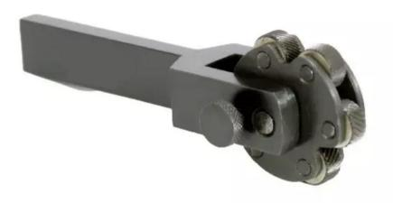
188.2 Total Length: 183 mm ± 3 mm Width: 188.3 28 mm ± 1 mm 13 mm ± 2 mm 188.4 Thickness: 188.5 Knurls Diameter: 19 mm 188.6 Fine Pitch: 0.8 mm 188.7 Medium Pitch: 1 mm 188.8 Coarse Pitch: 1.8 mm 188.9 Body Material: Mild Steel 188.10 Hardness: 55 - 60 HRC
