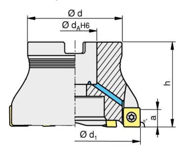
130.2 Type of Cutter: Right hand 130.3 Diameter (d1): 125.0 mm 130.4 Diameter (d): 88.0 mm 130.5 Bore Diameter (da): 40.0 mm 130.6 Thickness (h): 63.0 mm 130.7 Max RPM: 9800 130.8 Number of Pockets (Z): 12 Numbers
